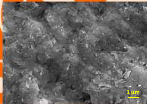
SEM image of the top view of the coating: heterogeneous deposits of the nanoflakes.
