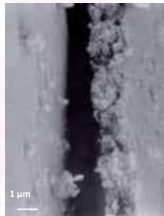
✓ General view of the coating & C/LiNi_{0.5}Mn_{1.5}O_4 film micrograph
